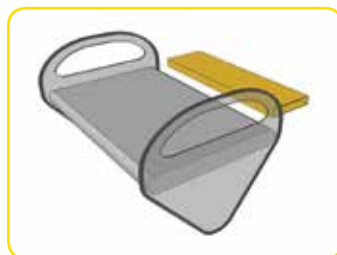
Bottom Overlap Wrapped Sleeve to Shrink Tunnel
